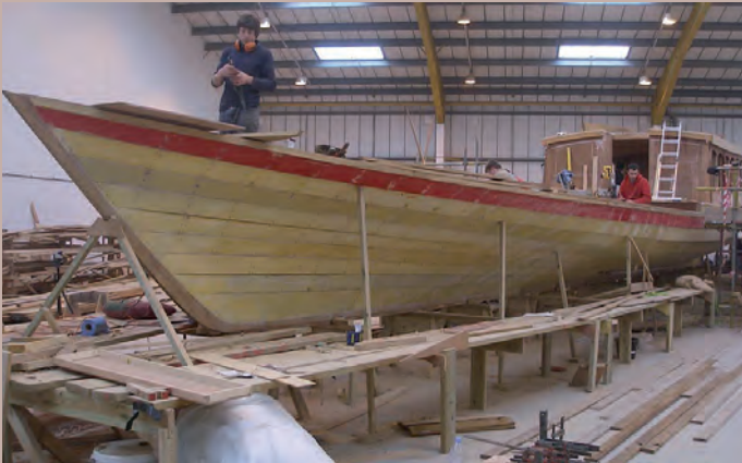
Air-dried Sweet Chestnut supplied to Richmond Bridge Boathouses for the royal rowbarge Gloriana
