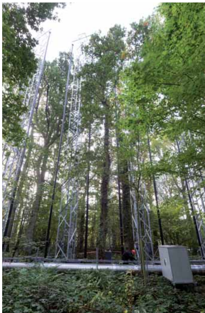
One of the six arrays; the black pipes take the CO 2 up to the point of release
