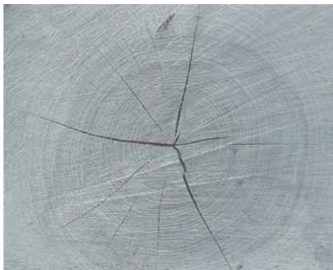
Star shake in the cross section of an Oak log
